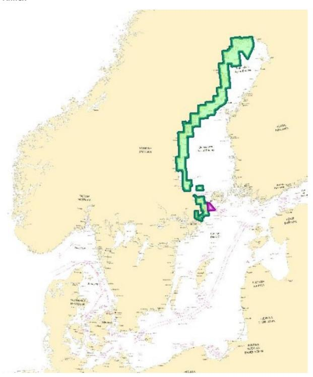
Example of ENC Approach from Sweden (updated 2021-06-21): Green cells are referring to the new chart datum BSCD2000, purple cells are ongoing adjustments to BSCD2000 and the rest of the cells refer to various Mean Sea Level.
